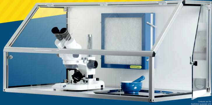
At 1000mm wide the SA1000 now gives ample space for both sample preparation and microscopy in the same simple enclosure.
